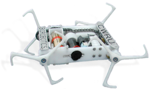
Figure 1. MiniWhegs IV robot designed by the Biologically Inspired Robotics Lab at Case Western Reserve University 1
