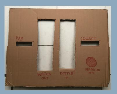
A prototype of the interaction section of the Clear Water Machine (left) was made to gain insights into how customers would use the machine to withdraw water. This interaction was prioritised, as the ease of use will determine the frequency that the machine is used, and therefore the amount of plastic bottle waste ultimately reduced.
